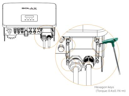
Step 6. Tighten the waterproof fastening head.
