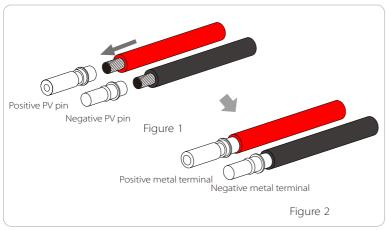
Step 4. Tighten the PV pin needle and the wiring harness to make the connection tight without looseness
