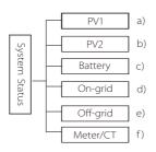
System status contains six content:PV1/PV2/Battery/On-grid (energy feed into or buy from the grid)and Off-grid and so on. Press up and down to select, press "Enter" to confirm the selection, and press "ESC" to return to the menu.
