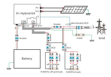
Diagram D: Neutral line and PE line are combined together, all loads connect to the Off-grid port;(Apply to Australia)
