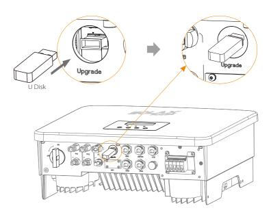
Step 3. LCD operation, enter the upgrade interface "update", as shown below(a): Please press the up and down keys to select ARM, then press down to set "OK", press the enter key to enter the software version interface:
