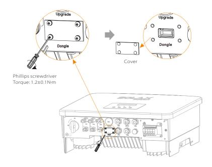
Step 2. Plug the Pocket WiFi Plus into the DONGLE port, use the screws in the Pocket WiFi Plus accessory to tighten it.
