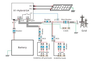
Diagram B: Neutral line and PE line are separated from each other, all loads connect to the Off-grid port; (For most countries)
