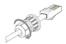
Step 5: Finally, find the corresponding COM, METER, CT, DRM, LCD poets on the inverter and insert the communication cable into the corresponding ports.
