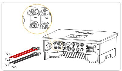
Schematic diagram of the inverter PV connected.
