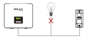
Figure: Wrong connection of load and inverter
