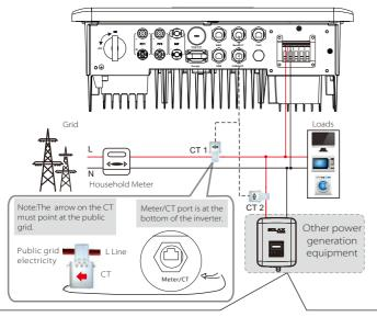
If the user has other power generation equipment (such as inverter) at home and wants to monitor both, X1-Hybrid G4 inverter provides CT2 communication function to monitor the power generation equipment.
