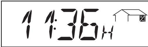
**operating hours** ... duration of operation of FRONIUS IG unit (HH:MM)
