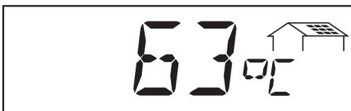
\* **module temperature** ... temperature at solar modules (degrees centigrade; can also be set for degrees Fahrenheit; temperature sensor No.1; sensor card optional)
