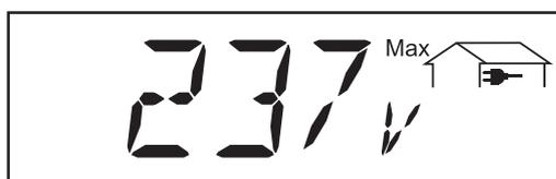
**Maximum mains voltage ...** highest reading of mains voltage (V) during observation period
