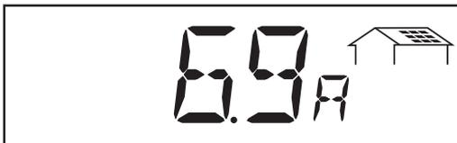
**module power** ... power supplied by solar modules at the moment of data display (Ampere)
