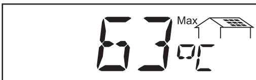
\* **maximum temperature at module...** highest temperature reading at solar modules during observation period (°C; can also be set for °F in setup menu; temperature sensor No. 1; applicable for sensor card)
