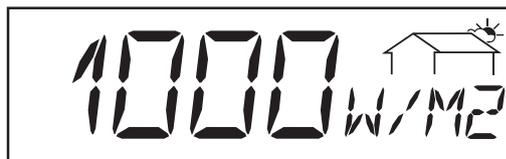
\* **insolation** ... insolation power output impact per square meter (Watt/m<sup>2</sup>; sensor card option)
