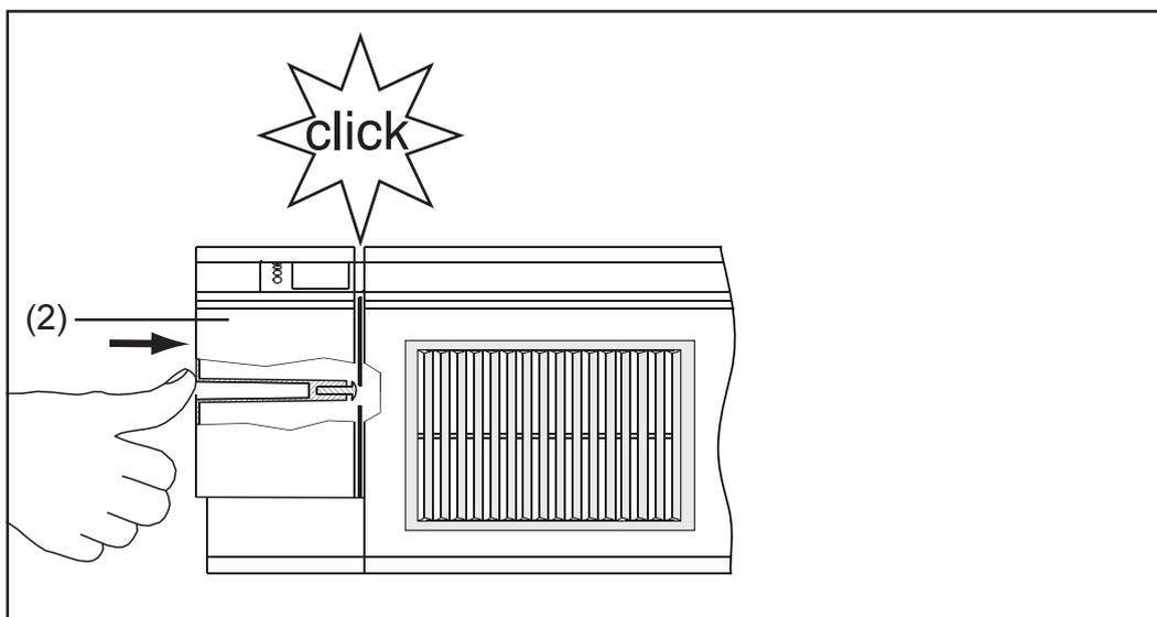
**Important!** To close the connection area put on cover (2) and push it forward until it reaches the locking position.
