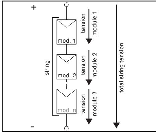
Power output and voltage are increased by combining a number of solar cells. If solar modules are connected in series like on a string, both the output potential as well as the voltage will increase.
