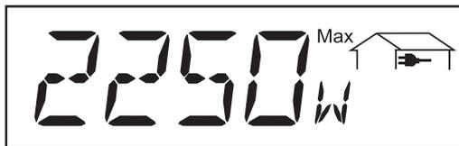
**Maximum power input ..** highest power input into main during observation period (W)
