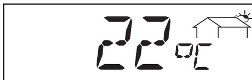
\* **ambient temperature** (°C; °C; can also be set for °F in setup menu; temperature sensor Nr.2; sensor card optional)
