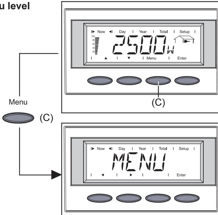
From the menu level you enter the display mode or the setup menu. Move into the menu surface by pressing key (C)
