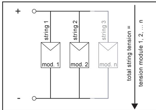
In a parallel connection of several such strings the potential output and the modular electric power will increase, while the voltage will remain unchanged. The total of all solar modules connected parallel and in series is called solar generator.
