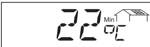
\* **minimum temperature at module...** lowest temperature reading at solar modules during observation period (°C; can also be set for °F in setup menu; temperature sensor No. 1; applicable for sensor card)
