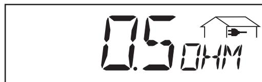
\* **mains impedance** ... resistance of mains - parameter for safe power supply to mains (Ohm; optional ENS)
