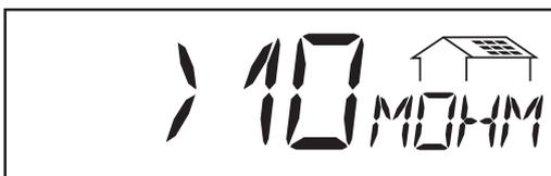
**isolation resistance** of photovoltaic generator (MOhm)
