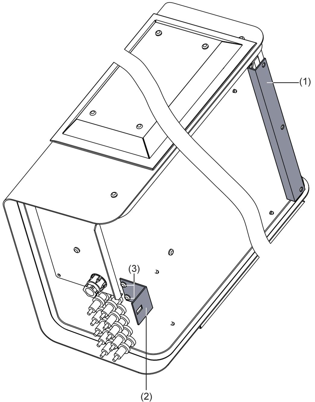
**Fixing the wall mounting frame for FRONIUS IG Outdoors**
