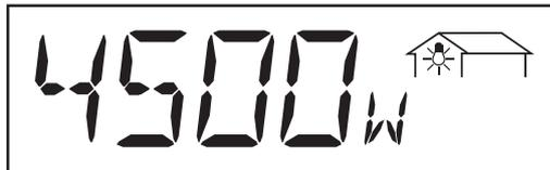
\* **power output drawn from mains supply...** present consumption (Watt; sensor card optional)
