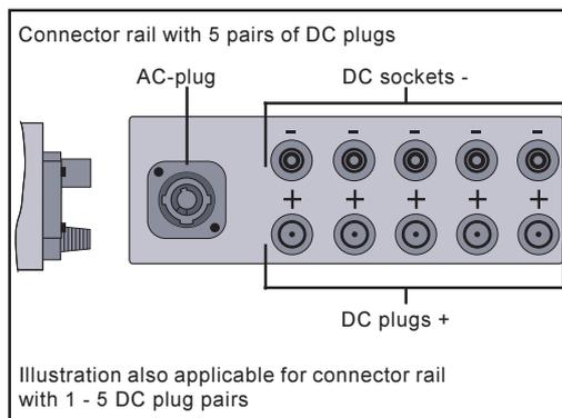
**Note!** When installing DC connections for solar modules make sure that the plus and minus poles correspond with the respective symbols.
