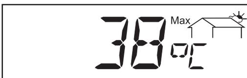
\* **maximum ambient temperature ...** highest temperature reading during observation period (°C; can also be set for °F in setup menu; temperature sensor No. 2; applicable for sensor card)
