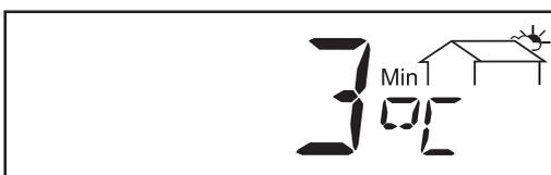
\* **minimum ambient temperature...** lowest temperature reading at solar modules during observation period (°C; can also be set for °F in setup menu; temperature sensor No. 2; applicable for sensor card)
