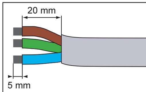
Bare the mains cable as shown in the illustration for the AC-plug-type connector
