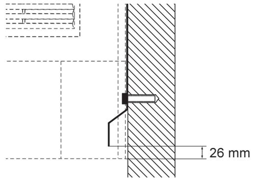
**Fixing the wall mounting frame for FRONIUS IG Outdoors**
